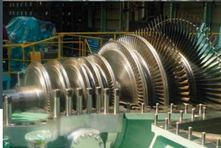
23,500kW Condensing Turbine for Sinter Cooler Waste Heat Recovery Power Plant, Visakhapatnam Steel Plant (VIZAG Steel)
