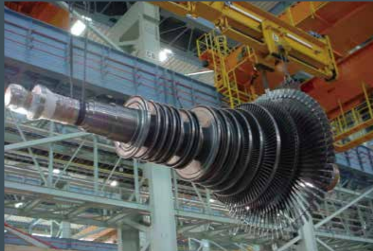
74,000kW Extraction (bleeding) Condensing Turbine for Blast Furnace Gas-fired Power Plant, West Japan Works of JFE Steel Corporation
