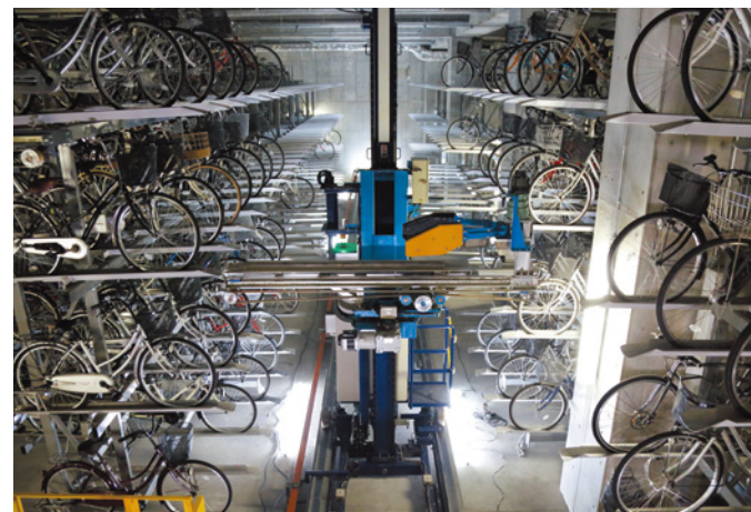
The low-footprint CycleTree® automated parking system outside Sagami-Ono Station (Kanagawa Prefecture).
