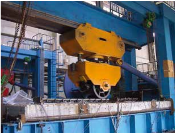
Periodic moving wheel load test
