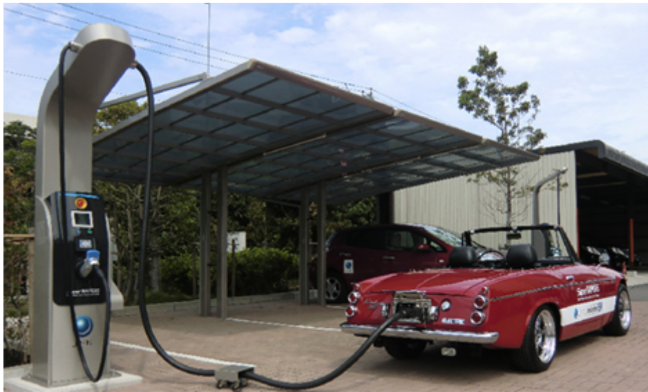
Test vehicle during super rapid charging
